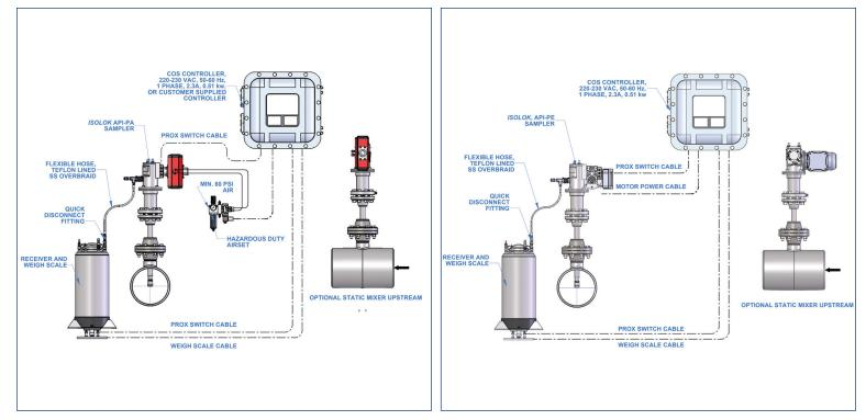
Sentry ISOLOK API-PA probe sampler Used in-line | Pneumatic actuator Sentry ISOLOK API-PE probe sampler Used in-line | Electric actuator
