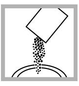
**3.** Add the contents of one Molybdate Reagent Powder Pillow for High Range Silica to the sample cell.
