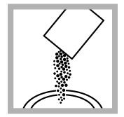
**5.** Add the contents of one Acid Reagent Powder Pillow for High Range Silica. A yellow color shows if silica or phosphorus is present in the sample.
