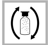
**4.** Quickly invert the AccuVac Ampul several times to mix.
