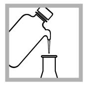
**6.** If the sample volume is less than 100 mL, dilute to approximately 100 mL with deionized water.
