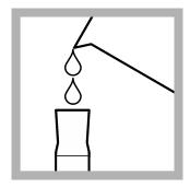
**4.** Use a graduated cylinder or pipet to measure the sample volume from Table 1 on page 4.
