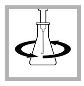
9. Put the end of the delivery tube fully into the solution. Swirl the flask. Turn the knob on the Digital Titrator to add titrant to the solution. Continue to swirl the flask. Add titrant until the color changes to light pink and stays pink for 30 seconds. Record the number of digits on the counter.
