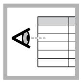
1. Select a sample volume and titration cartridge from Table 1 on page 4. For base determinations, use a Hydrochloric Acid or Sulfuric Acid Titration Cartridge.
