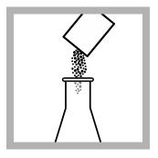
7. Add the contents of one Phenolphthalein Indicator Powder Pillow. The indicator is not necessary if a pH meter is used.
