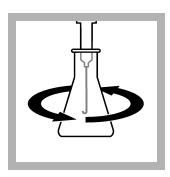
9. Put the end of the delivery tube fully into the solution. Swirl the flask. Turn the knob on the Digital Titrator to add titrant to the solution. Continue to swirl the flask. Add titrant until the color changes from light pink to clear. Record the number of digits on the counter.
