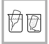
2. Prepare the blank: Pour at least 40 mL of ozone-free water in a 50-mL beaker. Fill an Indigo Ozone Reagent AccuVac Ampul with the ozone-free water. Keep the tip immersed while the Ampul fills fully.
