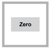
7. Push **ZERO**. The display shows  $0.00 \text{ mg/L O}_3$ .
